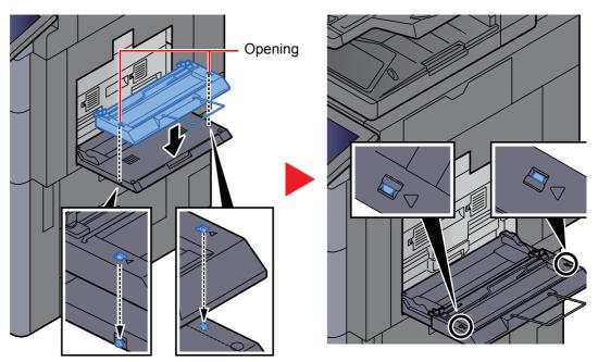
Fit the openings on the sides of the banner tray onto the tabs on the sides of the multipurpose tray, and press into place.
