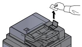
Clean the slit glass surface and the reading guide.
