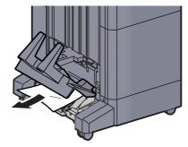
Press the release lever to pull the folding unit out.
