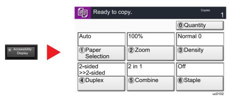
You can also control the screen using the numeric key corresponding to the number in circle. (Example: Press the [2] key on the numeric key pad to zoom.)
