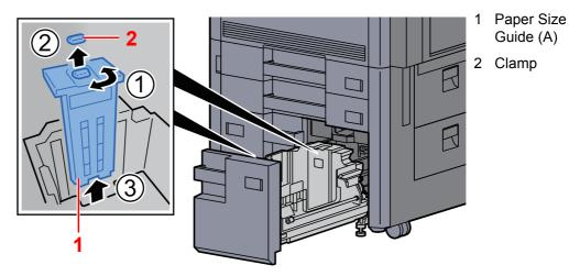
2 Insert the Paper Size Guide (A) into the slot (bottom of cassette) for the paper size to be used.
