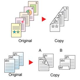
Produces two-sided copies from one-sided originals. In case of an odd number of originals, the back side of the last copy will be blank.
