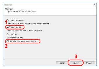
Selecting the [Overwrite settings on target device] checkbox will overwrite the machine's Address Book from entry No.1.
