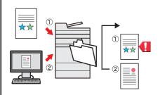
When paper empty error occurs at the cassette by specifying the special paper size or type, the machine skips the error job and perform the next job.
