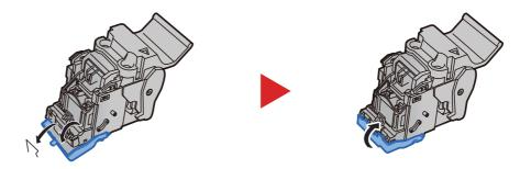
5 Install the Staple Cartridge Holder (B) or (C).
