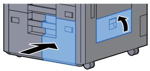
7 If the optional side feeder is installed, return the side feeder to the original position.
