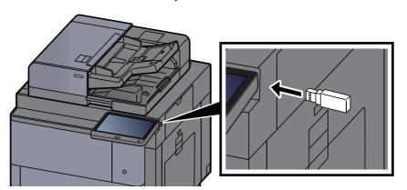
When the machine reads the USB drive, "USB Drive is recognized. Displaying files. Are you sure?" may appear. Select [Yes] to display the USB Drive screen.
