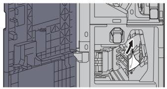
Remove the Staple Cartridge Holder (B) or (C).
