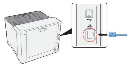
**2** Connect the other end of the cable to the hub or the PC.
