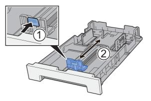
**3** Adjust the position of the paper width guides located on the left and right sides of the Cassette 2.
