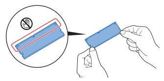
To protect electronic parts, discharge static electricity from your body by touching a water pipe (faucet) or other large metal object before handling the memory modules. Or, wear an antistatic wrist strap, if possible, when you install the memory modules.
