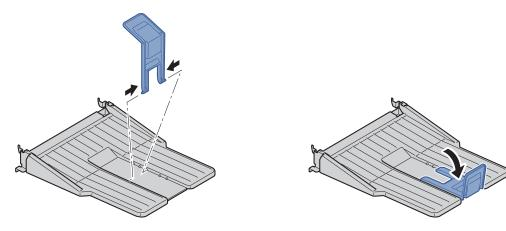
Install the rear tray on the rear of the machine.
