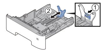
3 Attach the auxiliary guide to the paper length guide as shown in the illustration.
