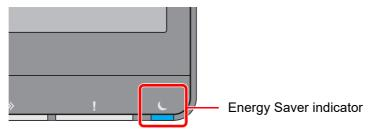
If print data is received during Sleep, the machine automatically wakes up and starts printing. Also when fax data arrives while the machine is in Sleep, the machine automatically wakes up and starts printing.
