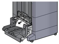
Open the folding unit conveyor guide.
