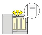
When reading a document from the document processor, if the multiple feeding of documents is detected, then the reading stops automatically.
