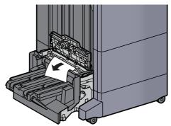
11 Open the folding unit conveyor guide.
