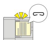
When reading a document from the document processor, if a stapled document is detected, then the reading stops automatically.
