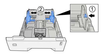
2 Adjust the paper length guide to the paper size required. Press the paper length adjusting tab and slide the guides to the paper size required.
