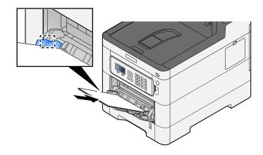
Insert the paper along the paper width guides into the tray until it stops.
