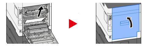
**3** Open the Rear Cover 2 and remove the jammed paper.
