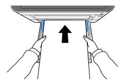
After printing starts, catch the paper when it is output so that it does not fall out of the tray. When using the inner tray as the output location, do not stand up the stopper.
