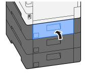
**3** Open the Rear Cover 3 and remove the jammed paper.
